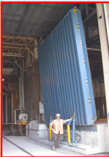
20' X 20' 30,000 POUND CAPACITY DUAL LANE RAIL BRIDGE
