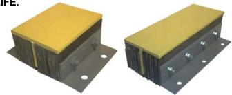
THE FLAT REINFORCED STAMPED RUBBER SECTIONS ENSURE EVEN SUPPORT TO PREVENT DENTING. THE WRAP AROUND FRONT FACE KEEPS THE RUBBER IN PLACE, ELIMINATING A POTENTIAL 'MUSHROOMING' EFFECT.
