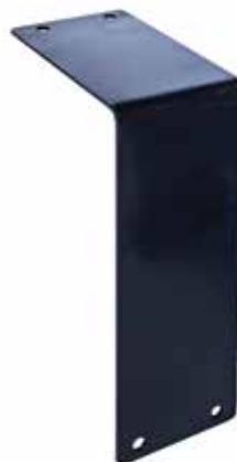
EXTENSION BRACKET Used when the dock bumper projection must be increased and it cannot be accomplished by choosing the bumper size of appropriate projection. They can also be used to extend an existing bumper to the proper projection. Extension brackets can ship with the dock bumpers welded to them for easier one-step installation.*
